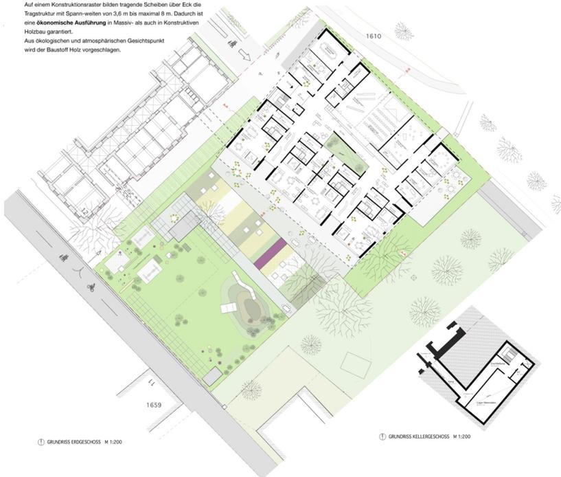
① GRUNDRISS ERDGESCHOSS M 1:200
